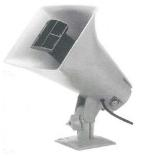
**Features:** Designed for noise penetration and speech clarity; excellent sensitivity as a microphone in two-way systems; weather and corrosion resistant construction using stainless steel fasteners and UV resistant thermoplastics; conservatively rated at 16 Watts continuous duty; diffuser suppresses on-axis hot spots.
